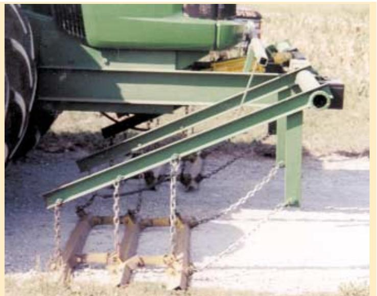
Pivoting frame bolts to side of tractor frame. A single hydraulic cylinder lifts "stalk stompers" up when they're not needed.
