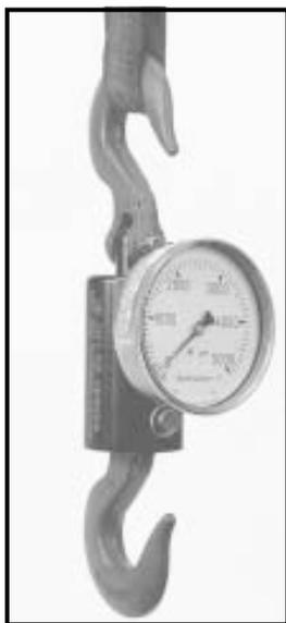
With a hook at either end, hydraulic scale can be suspended from a block and tackle, front-end loader bucket, or forklift blade.
