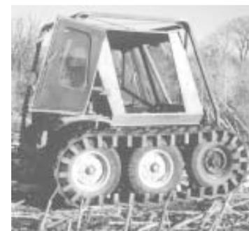
**Rig's tracks are friction-driven by three sets of axles equipped with 15-in. tires.**
