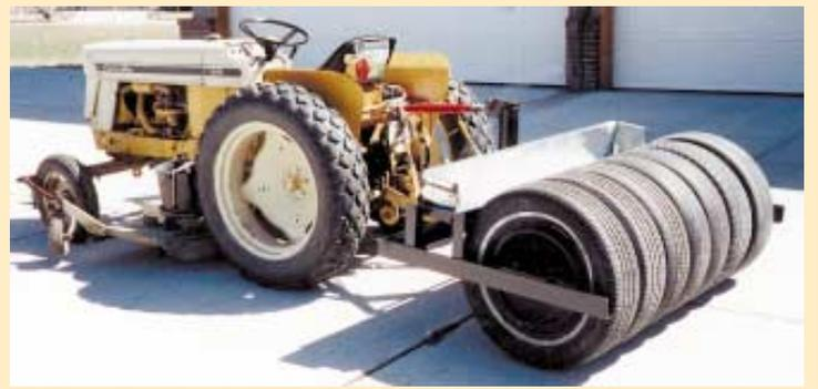
Mueller pulls rubber-tired roller behind tractor when mowing. Weed seeds with burs stick to wheels and are collected in hopper for disposal.
