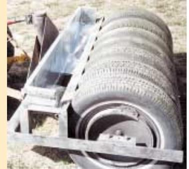
Weed seeds are disposed of through hole in center of hopper.
