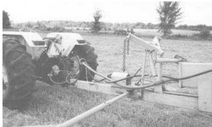
**Note pto-powered hydraulic pump on tractor and hoses running back to oil reservoir.**
