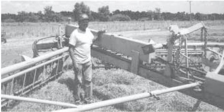
**Bob Sell equipped his tractor with a pto-powered hydraulic pump and mounted a 20-gal. reservoir and cooler directly on the hitch of his R-23 Vermeer Twin Rake.**
