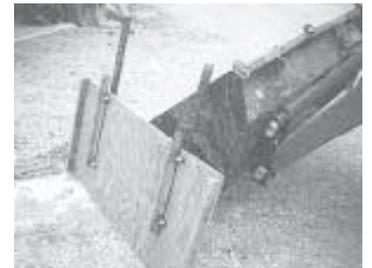
Lawson cut up steel T-posts to make mounting brackets that slip onto bucket.
