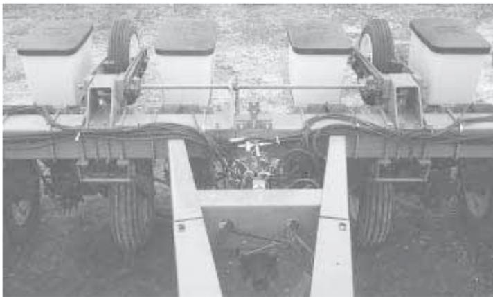
Wheel-drive kit gets drive chains up and out of the trash and dirt, and eliminates the need for drive chain disconnects.
