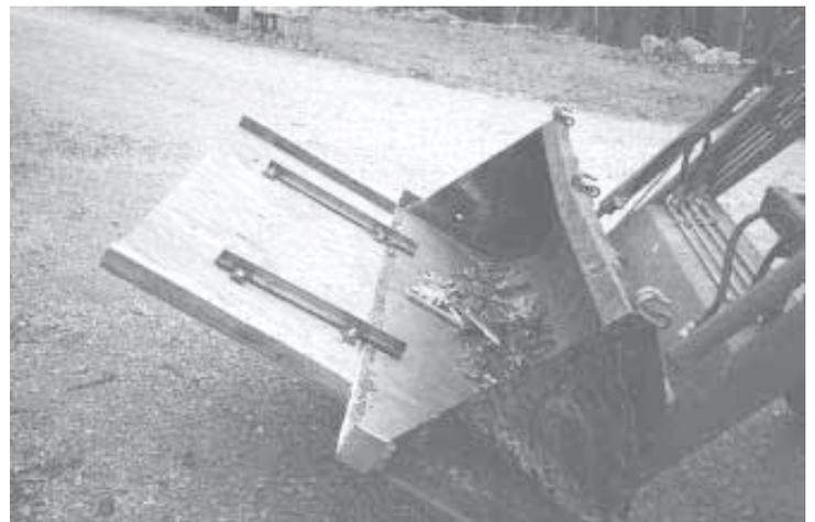
Wooden platform slips on over lip of bucket, more than doubling its carrying capacity.
