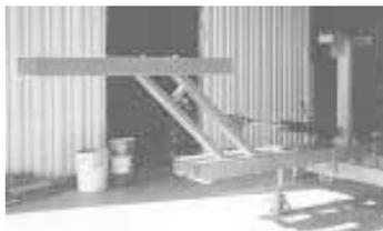
Frame is built from 7 by 7-in. steel tubing. A 5-in. cylinder on each side provides the lifting power.
