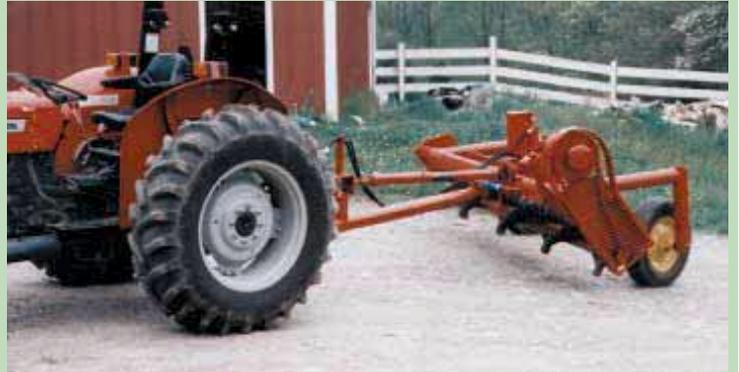
Teeth for the auger-shaped rake are spaced around a 4-in. pipe. They pick up and windrow rocks up to 10 to 12 in. in size.
