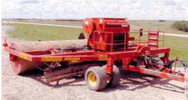
The 20-ft. wide "roller blader" is equipped with a pair of 10-ft. "swing blades" that can be angled forward or backward. Gauge wheels on front and back keep blades level.
