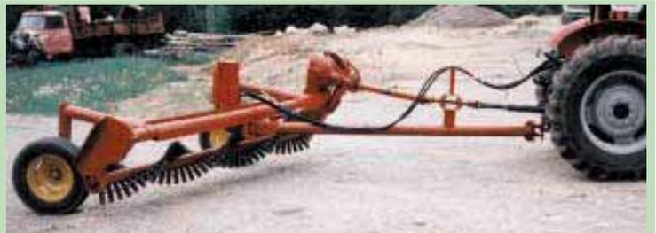
Geer built this rock rake using parts from an old New Holland Super 66 baler.
