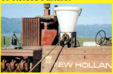
La Macchia injects clover and other grass seed into bale chamber as he bales. A pair of rubber tubes run from hopper through holes cut into baler.
