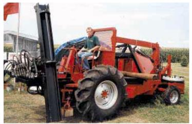
Up-front post driver tilts hydraulically in any direction and mounts on a telescoping table that extends 3 ft. out to the side and 3 ft. to the front.
