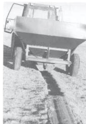
Bottom unloading wagon pours fill material into rut. A blade scrapes down ridges on both sides of rut and levels fill material as wagon passes by.
