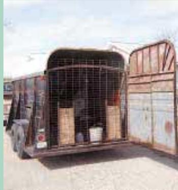
Inside trailer's back door Ruby installed a gate made from a cattle panel. Two narrow wooden doors built into gate can be raised to allow dogs to leave trailer for exercise.
