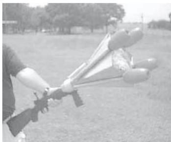
Net is packed into canister between the four barrels of gun.
