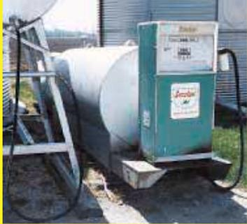
tion gas pump mount on a pair of large steel skids. It can be used on the farm for normal refueling or taken to the field. **(C.F. Marley, Nokomis, Ill.)**
