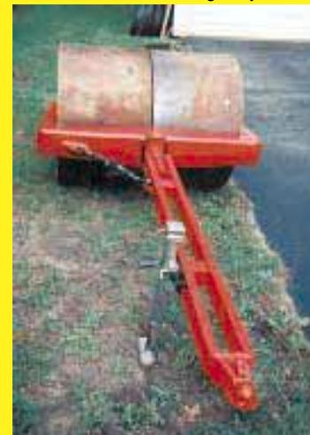
king pin, welding a 6-ft. drawbar to the kingpin. I used a 2 5/16-in. ball hitch to add flexibility when towing. I put a ratchet jack from the yoke to the drawbar to enable us to offset the roller to reach past the tractor wheel. The roller wheel is 50 in. wide and 40 in. high. **(George Wojnar, 5 Malsbury Lane, Cream Ridge, N.J. 08514 ph 609 758-7295)**
