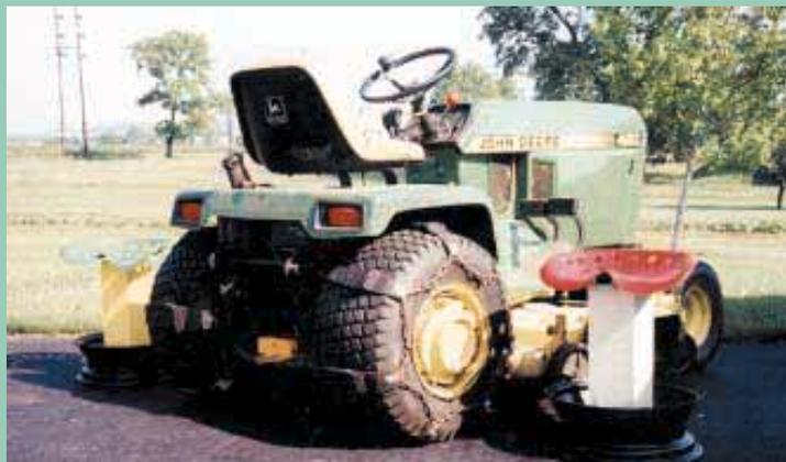
I made "chains" for my garden tractor out of rubber tires. I just cut strips out of a car tire and bolted them to lengths of chain that wrap around the sides of the tire. The rubber strips are a couple inches wide and lay flat on the tire, giving you extra traction without ripping up the ground. Great on steep hillsides when
