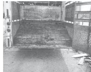
**Trailer is designed to load cattle from the ground, with no need for a loading chute.**
