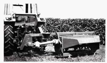
Taarup Belt Mower/Conditioner has a new linkage design that allows it to swing up and backward when it hits an obstacle, and then turn automatically forward again to working position without any stop.
