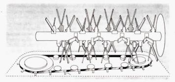
Mower's cutterbar is a rotating V-belt with 29 attached, replaceable knives. Conditioner rotor is located above cutterbar.
