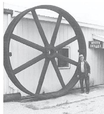
Winter stands beside a 12-ft. dia. rope pulley off a 150 hp. steam engine. At one time it was used by a grain elevator to run a generator, grain mill, and line shaft.
