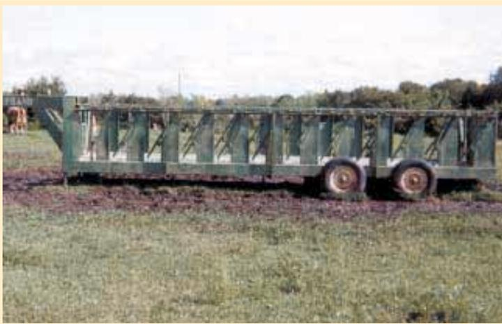
Yarbrough's 30-ft. long feeder is designed to feed big round bales as well as silage or grain. Cattle are held by self-locking gates on the sides, front and rear of wagon.
