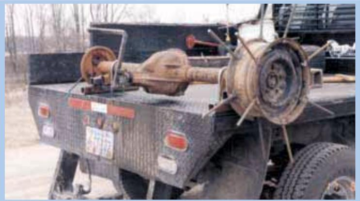
Wire roller bolts to truck flatbed. It consists of a car rear end with a wheel and rim attached to one of the hubs. Lengths of 6-in. rebar are welded to each side of rim.
