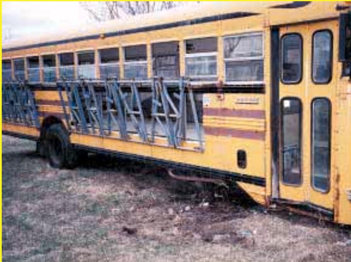
Multiple self-locking headgates cover holes cut into side of bus. After driving out to pasture, Kerr dumps grain onto floor in front of each headgate to catch cows.
