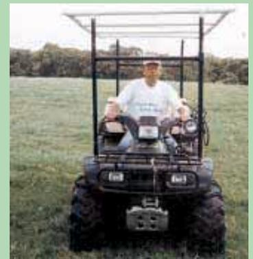
"Sun roof" is made from a PVC frame covered by a close-weave fiberglass cloth. tank and from having no support.
