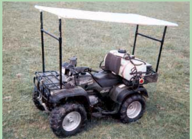
T.C. Mallett says the "sun roof" he built for his 4-wheel ATV provides great protection from the hot Texas sun. Note homemade back seat rest on spray tank.
