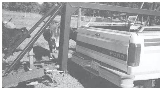
Fifth wheel hitch has a ball hitch built into it, allowing Cooper to quickly switch from one trailer to another.
