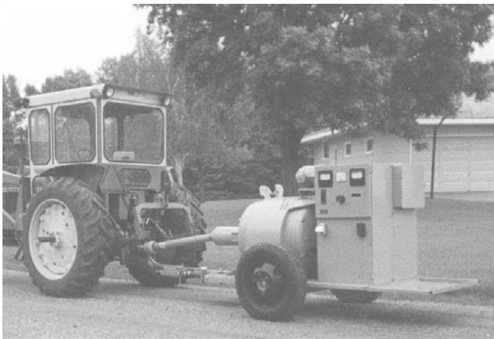
Ellsworth Olson and Meredith Ulstad converted a 100 hp, 3-phase synchronous electric motor into a pto-powered backup generator.
