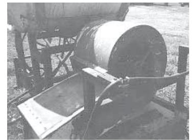
Pto-driven crop mister uses a furnace fan to apply foliar fertilizer to soybeans. Blower can be rotated up to 200 degrees in either direction using a hydraulic cylinder.
