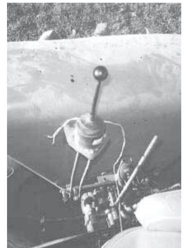
Davies uses a "joystick" to control the extra hydraulic outlets.
