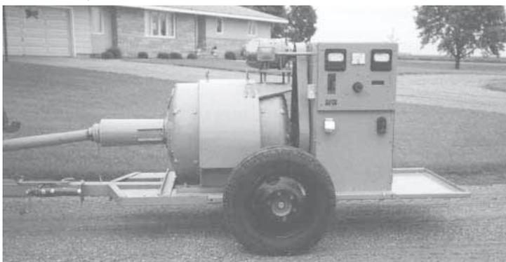
Olson made generator trailer from the front axle of a 3/4-ton pickup.
