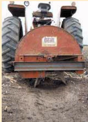
He cut off about a third of the blower and then built a heavy angle iron frame around it. Blower fan digs a shallow ditch about 20 in. wide and 5 to 6 in. deep at center.
