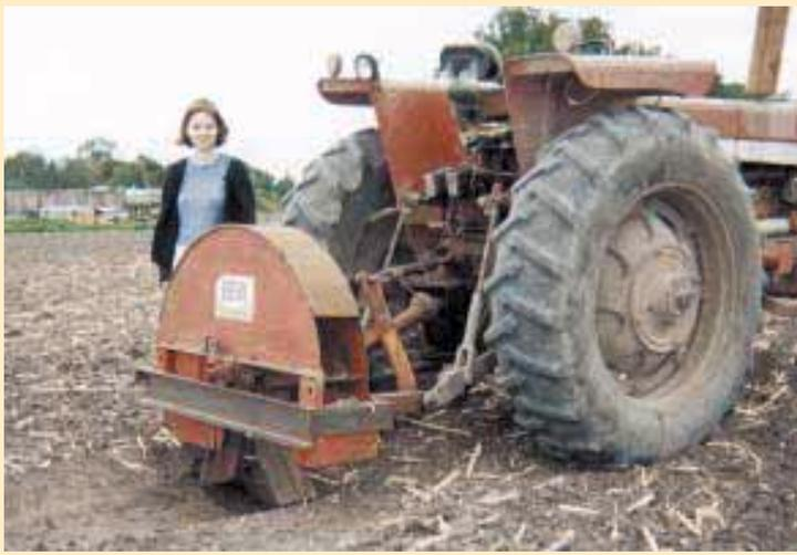
Elwin Harder spent less than \$100 to make this ditcher out of a Gehl silage blower.
