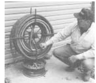
four U-shaped rods to an old spoked implement wheel. The hose reel mounts on a stand made from an auto wheel with an upright pipe that bolts to the hub on the spoked hose reel wheel.
