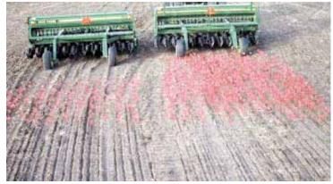
These two Deere 750 drills were pulled out of the ground at the same time. Drill on the left was equipped with the Seed Mizer attachment; the drill on the right did not have it. Flags mark seed left on the ground by each drill. There are 1,490 flags on the right but only 452 flags on the left.
