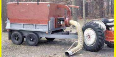
Trailer is equipped with a commercial leaf blower which pulls leaves through a 12-ft. long hose and into the box.
