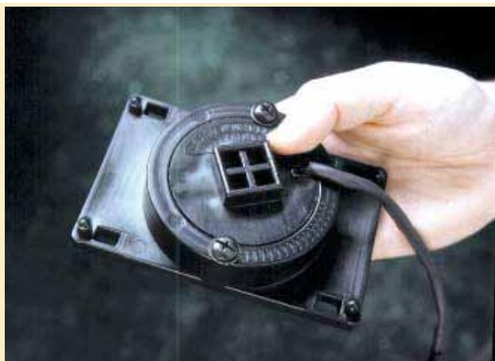
“Spray Saver” straps onto rocker arm of tractor and contains a 10-amp mercury shut-off switch. It'll control up to three direct-to-valve solenoid switches at one time.
