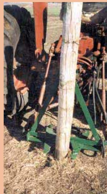
Unit is equipped with hydraulic-operated jaws that clamp onto post. The 3-pt. does the lifting.
