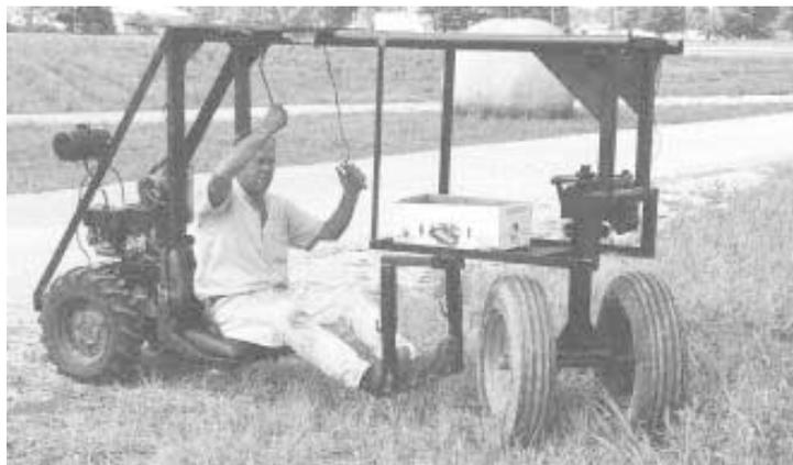
Gears on McKee’s “strawberry picker” are shifted with an overhead connecting linkage.
