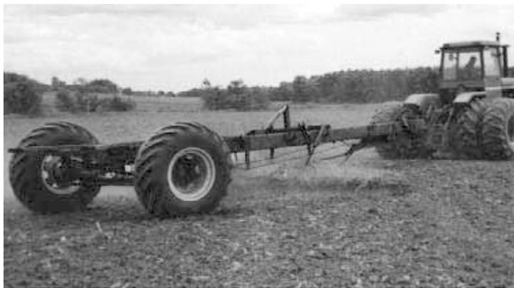
Robert Davis built pull-type land leveler by welding a pair of semi tractor frames together end to end. He pulls it with a Deere 8440 4-WD tractor.
