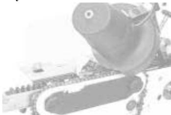
**One cam feeds the chain along while the other oscillates the grinding head up and down.**
