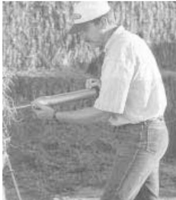
**Hay sampler has an easy-to-use "push-in" probe that cuts a core 5/8-in. in diameter and 18 in. long.**
