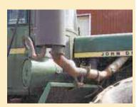
Muffler now mounts on a 90° exhaust elbow which Davis bought new from Deere.
