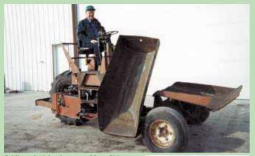
Juhl's rock picker is powered by a 50 hp. Isuzu diesel engine and has a hydrostatic transmission and power steering. The 3-wheeled rig has a single rear drive wheel and two smaller steering wheels up front.
