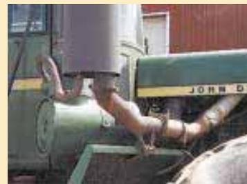
Muffler now mounts on a 90° exhaust elbow which Davis bought new from Deere.
