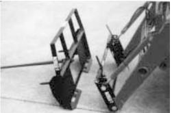
Hitch consists of two parts. One part pins onto loader mounting brackets and the other pins onto the attachment
