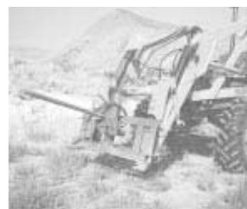
Hydraulic-driven, heavy-duty bale unroller quick-taches to front-end loader on Swanson’s Deere 2940 tractor.
