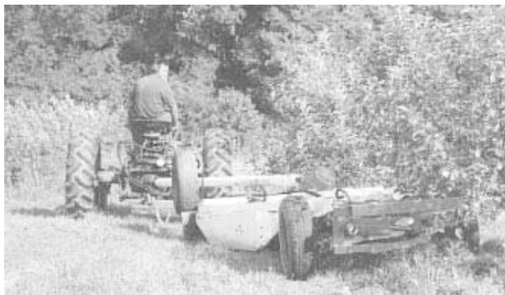
Rear-mounted steering axle allows Wickham to swing mower 5 ft. to either side of tractor to cut weeds between trees in his orchard.
