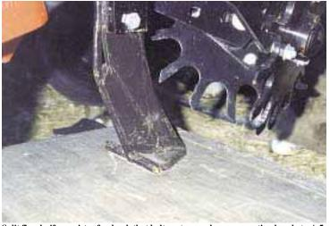
Split flow knife consists of a shank that bolts onto row cleaner mounting brackets. A 5in. wide sweep welds to bottom of shank. A fertilizer tube runs along back side of shank down to sweep where the tube splits to deliver fertilizer directly behind the point.
