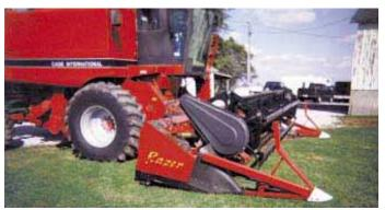
Loftus mounted his high speed patented chain-type cutterbar on his Case-IH 1660 combine equipped with a 20-ft. grain platform. He calls it the "Razer".
