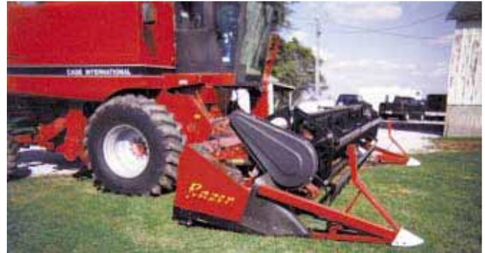
Loftus mounted his high speed patented chain-type cutterbar on his Case-IH 1660 combine equipped with a 20-ft. grain platform. He calls it the “Razer”.
