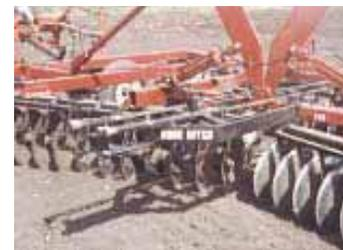
“Sure Hitch” clamps onto a toolbar and consists of a spring-loaded pin, guide assembly, and drawbar. Drawbar can be pulled backward 15 in. and swung 15 in. from side to side.
