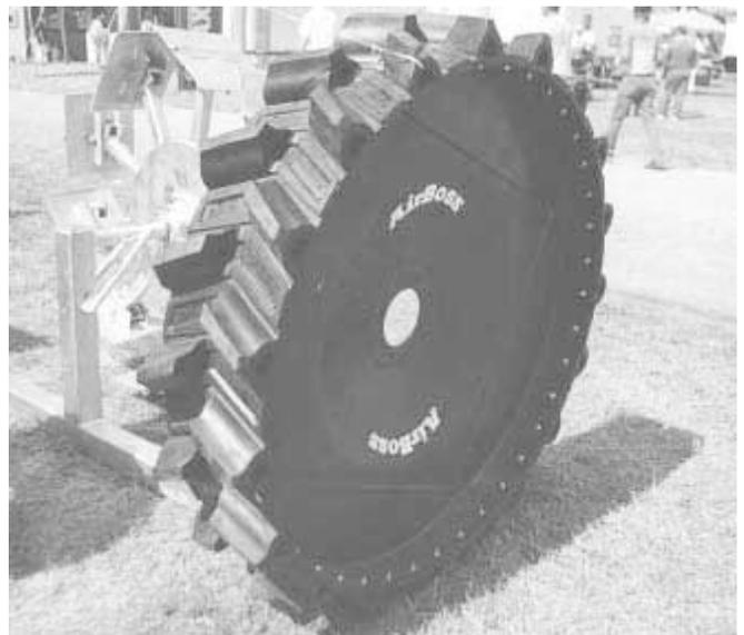
Tire consists of hollow rubber segments bolted onto a special-made steel wheel.
