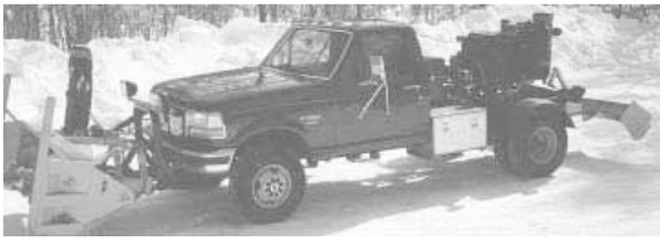
Pickup is equipped with 7 1/2-ft. snowblower on front and 6 1/2-ft. snow blade on back.
