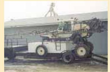
Melroe sprayer drives right up onto trailer fenders for transport, riding above the water tank.
