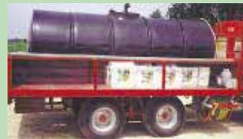
Rear 25-ft. deck supports a 1,600-gal. poly water tank, with storage compartments on each side of it for chemicals.
