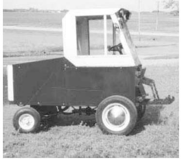
The 2-WD rig has a cab as well as a 3-pt. hitch and pto on front. Fisher used the bean rider's engine, seat, hydrostatic transmission, live hydraulics, power steering, fuel and hydraulic tanks, hydraulic hose, and battery.
