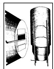
Feed bin was made by bolting an 80-gal. cone-shaped hog waterer into the bottom of a rusted-out 300-gal. fuel tank.
