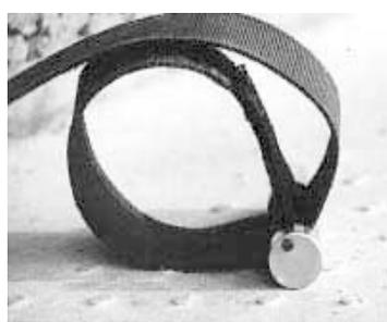
pin to join the two ends of the strap. It was sewn into the strap by a shoemaker. To use, he simply tightens the strap loop around the filter with a wrench, and keeps tightening until the filter works loose. Works great and never stretches out the way some commercial strap-type wrenches do.
