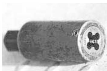
as manifolds. It consists of a 3-in. length of 1 in. dia. pipe with a 3/4-in. hex nut or shaft welded to one end and a small thread die fitted into the other. A 1/4-in. dia. set screw holds the die in place in the pipe. To use, he simply turns the die on the bolt with a socket or straight wrench. Works great on any size bolt from 3/8 up to 1/2 in., he says.
