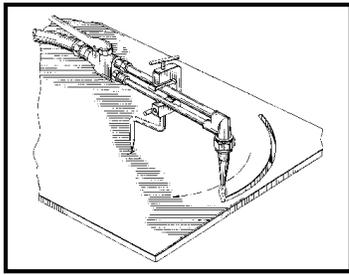
To make a circle, you stick the pointed end of the circle cutter into a dent made by a center punch.
