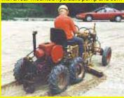
ponents. The blade raises up to 1 ft. off the ground, can be adjusted up to a 45 degree angle either way, and can be moved 1 ft. out to either side with a hydraulic sideshift I rigged
