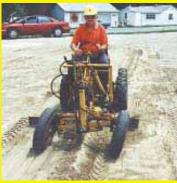
gine. I chose this engine because I had always wanted to hook up one of those old engines to a set of wheels just to see how it would work. The grader has a gearbox out of an old 6-speed Wheelhorse garden tractor transaxle. A V-belt off the engine drives a jackshaft which is fitted with a #40 roller chain that powers the transaxle. The tandem drive wheels are 12-in. tires off an old garden tractor.
