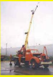
The semi tractor is a 1947 IH KS-8 I bought used in 1953 with between 150,000 and 200,000 miles on it. It's powered by an IH "Black Diamond" OHV in-line 6-cyl. 269 cu. in. engine that was overhauled in 1952 and hasn't been opened since.
