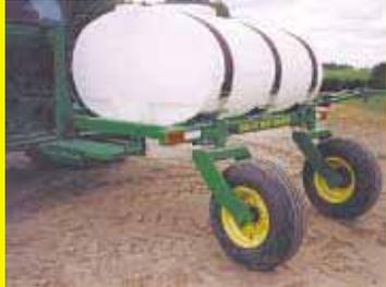
taking some of the weight off the assist wheels and reducing compaction. The wheels can be adjusted to fit 30 or 22-in. rows. Larger 750 and 1,000-gal. tanks are also available.
