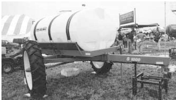
Note how wheels pivot on "steerable" hitch.
