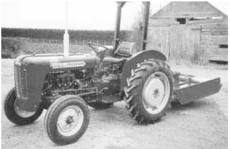
"Smallholder" tractors range from 30 to 55 hp and are based on Massey Ferguson 35 castings. They contain a mix of new and remanufactured parts that keeps cost down.
