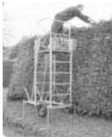
Scaffold platform moves upward at 1-ft. intervals to a maximum height of 7 ft.
