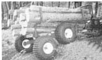
Compact design allows the timber hauler to travel easily over rough terrain.
