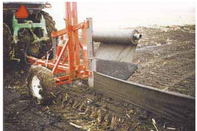
Pull-type fabric layer unrolls and buries a woven fabric that shores up erodable soils.
