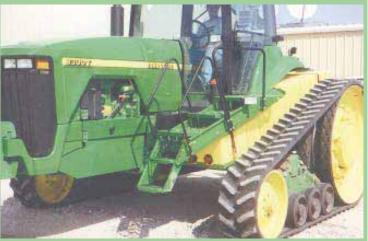
Tanks mount between tractor frame and tracks so they don't interfere with cab access and operator visibility. Each tank holds up to 260 gal. of liquid fertilizer or chemicals.
