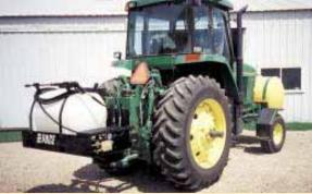
Unit also mounts on a tractor Cat. II hitch, using 3-pt. hitch adaptors that attach to the platform.
