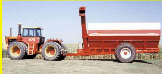
Gary Lantz wanted to use his 1979 Versatile 875 4-WD tractor to operate his 1,000-bu. Killbros. auger wagon. The tractor didn't have a pto, so he mounted a Chevy 350 cu. in. gas engine between the tractor's rear wheels.
