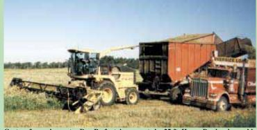
Custom forage harvester Dan Prefontaine mounted a 25-ft. Honey Bee header on his New Holland FX45 self-propelled forage harvester. Silage is blown into a 15-ton Jiffy "accumulator box" which unloads on-the-go into tandem axle trucks.
