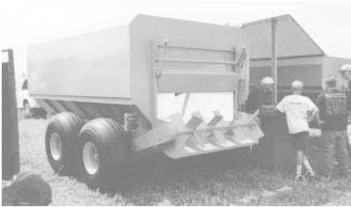
Spreader is designed to be hydraulically raised on-the-go. As it's raised, manure flows by gravity out the back into a pto-driven reel.
