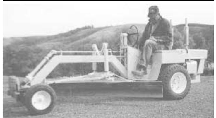
Fun-to-drive road grader is 6 1/2 ft. wide and 11 ft. long. It's powered by a 23 hp Kohler engine and is painted Caterpillar yellow.
