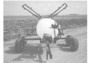
Tandem axle sprayer is equipped with a 5 hp Honda engine and available with either a 110 or 150-gal. tank.
