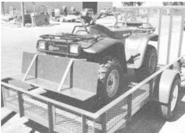
Steel deflector, bent to a 90 degree angle, mounts across front of ATV to deflect weeds.
