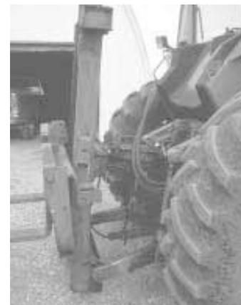
Obrecht mounted a forklift mast on the 3-pt.'s lower lift arms and mounted a hydraulic cylinder in place of the top link so he can tip the forks.
