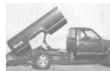
Bolt-on kit lifts box up to a 45 degree angle in 10 seconds with a maximum load.
